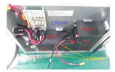
4. Please install the fuse board in battery case and connect it on the right point ,refer to the below circuit's link.
